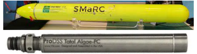
Fig. 3. Top: SAM UAV from SMaRC. Bottom: Total Algae sensor from YSI
