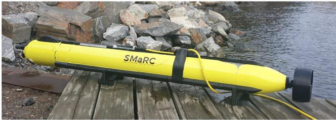
Fig. 8: The SAM AUV developed by SMaRC.
